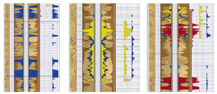
The log illustrates TBlockSure diverter distribution across multiple vertical formations using three proppant tracers, identified by blue, yellow, and red. The blue represents the first three stages, the yellow represents the middle three stages, and the red represents the final two stages.
