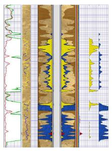
The log illustrates TBlockSure diverter distribution across multiple vertical formations using three proppant tracers, identified by blue, yellow, and red.
