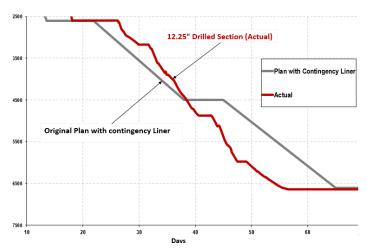
The rugged design of Weatherford's Magnus RSS delivers reliable, accurate, and fast operations as shown in this days vs depth comparison where the Weatherford solution increased ROP by 5% and saved 11 days of rig time.
