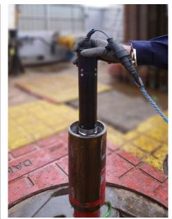
The tools power up and function checks are completed at the surface via an inductive coupling interface.
