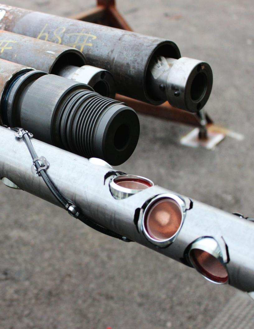
Four target intervals selectively perforated in a single run,
