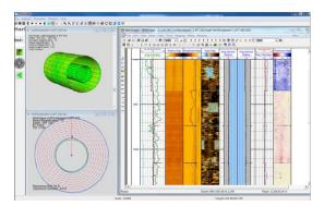
The UltraView tool delivers a comprehensive evaluation of casing, cement, and borehole fluid measurements. On the left is a log presentation from UltraView measurements. On the right, the same measurements from UltraView are used to generate interactive 2D and 3D images.
