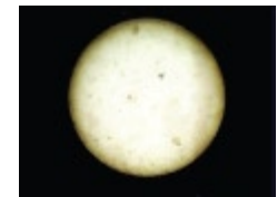
Microscopic image of fluid sample before Weatherford NAS filtration service (NAS Class 8).
