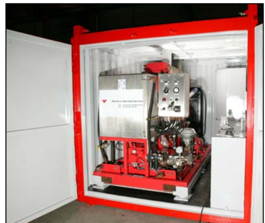
Weatherford's jetting unit was kept on standby in the event of unforeseen blockages.
