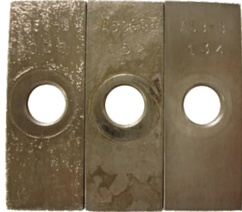
Three corrosion coupons from the comparative investigation in Weatherford's San Antonio lab: Results from use of uninhibited cryogenic nitrogen (left), uninhibited membrane nitrogen (center), and inhibited membrane nitrogen (right).
