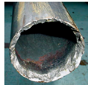
The RCT cleanly cuts all types of tubulars, without using explosives, making it one of the safest pipe-cutting devices available.
