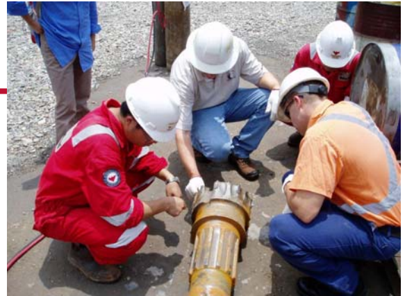
Weatherford engineers inspect a used air-hammer bit after it drilled over 3,281 ft (1,000 m) of hard formation.
