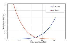
time-consuming, steady-state methods are highly reliable and allow for the determination of relative permeability at a wide range of saturation levels, even early in the life of the field.
