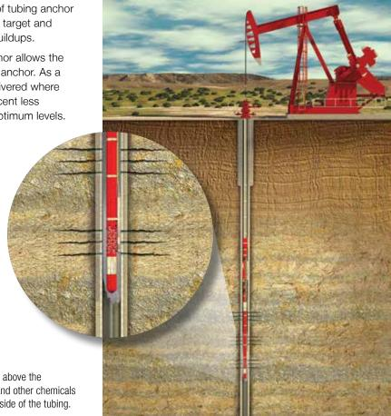
Weatherford's capillary tubing anchor is set above the rod pump and delivers foamers, inhibitors and other chemicals through a capillary string banded to the outside of the tubing.
