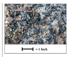
The 14.5-in. long Minima composite frac plug breaks down into small, manageable cuttings that pump to the surface for a quick cleanout.
