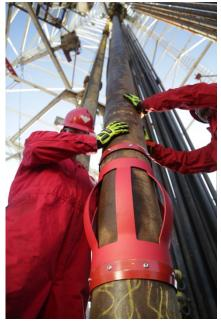
The Weatherford VariForm centralizer keeps starting and running forces at or near O lbf (O N) for minimum drag during casing running, and it achieves high restoring forces for maximum standoff during cementing operations.
