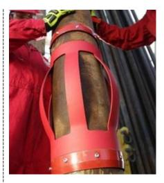
The one-piece VariForm centralizer slips easily onto liner or casing to provide a single, metallurigcally invisible weld with no hinges or mechanical connections. The bows collapse during run-in and then, upon landing, restore to the full outside diameter to provide reliable standoff.
