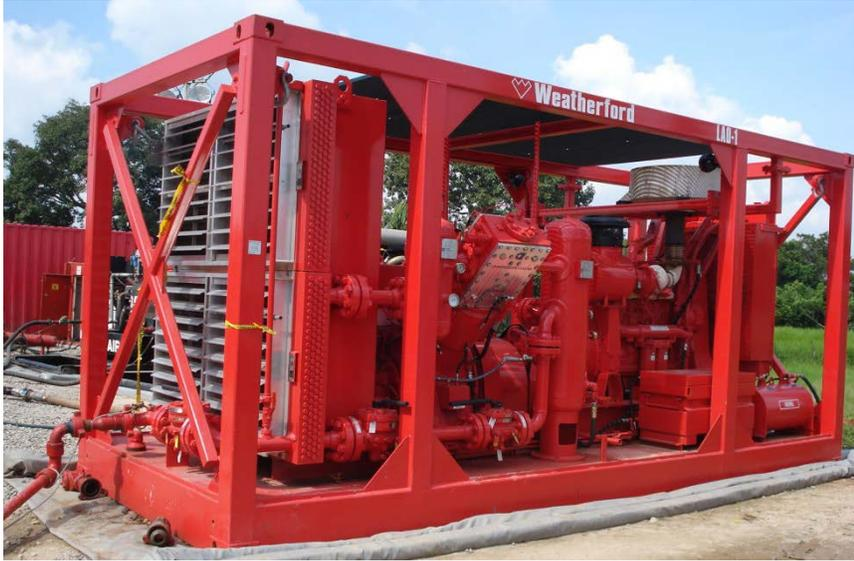
Weatherford performed UBD using a booster compressor (above) to mitigate mud losses and drill the section to TD. This type of compressor takes a high volume of gas at a low pressure—between 175 to 350 psi (1.2 to 2.4 MPa)—from the primary compressor and boosts it to a high pressure.
