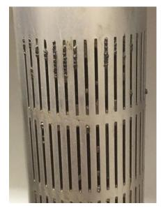
The above image shows the control-valve screen slot of the pulser used in the HPHT well. The screen is in excellent condition and successfully captured harmful, large components of the LCM to avoid blocking the control valve.
