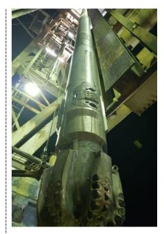
The Magnus RSS sidetracked off of a challenging cement plug in a single run.
