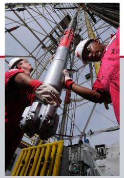
Weatherford's *RipTide* drilling reamer features RFID technology to enable on-demand activation and deactivation any time while drilling or tripping. The *RipTide* RFID model is the industry's first electronically controlled drilling reamer.
