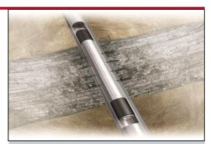
Two Weatherford MetalSkin liners were run to isolate multiple intervals in a well with years of decreased production. The successful MetalSkin installations significantly increased production rates and permanently isolated the water production zone. That success encouraged the operator to consider drilling additional wells in the Shirley field.
