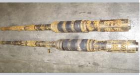
The functionality and durability of Weatherford's WRP bridge plugs—even after five years downhole—enabled this operator in Germany to quickly retrieve both plugs, preventing a long and costly fishing and milling operation.
