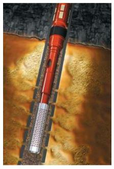
Weatherford provided a thru-tubing solution that included a high-rate squeeze gravel pack (shown above) in a well plagued by sand problems.
