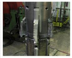
After successfully removing 100 ft (30 m) of 7-in., 29-lb/ft N80 casing, this section mill exhibited only 14% wear.
