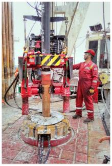
Operated with a simple push of a button, the Vero conventional system controls the makeup and evaluation of premium pipe connections on land and shallow-water rigs.
