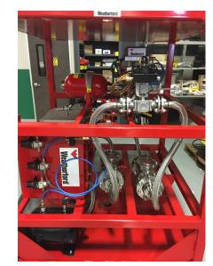
The control module of the MPD fluid-extraction system includes a PLC, which reduces sample pressure to less than 10 psi (0.07 MPa) for conventional gas-detection methods.
