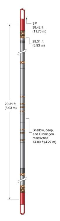
The Compact dual laterolog (MDL) tool provides accurate, realtime, deep-resistivity readings.
