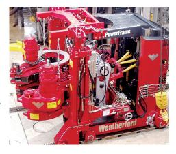
The tong is capable of fully mechanized remote operation or semimechanized operation and is compatible with the patented\* Weatherford PowerFrame<sup>®</sup> and PowerScope<sup>®</sup> tong-positioning systems.
