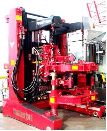
24-50 high-torque casing tong installed in the PowerFrame system
