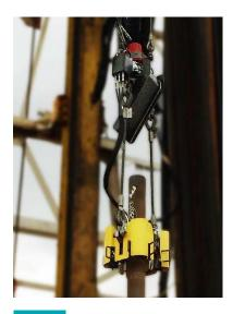
The flush-joint elevator eliminates the need to thread lift nubbins to lift and make up each joint.
