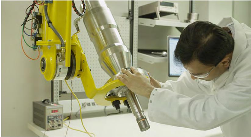
The award-winning Red Eye® Subsea Water-Cut Meter uses near-infrared light absorption technology to provide water-cut measurement, water-onset detection and water-to-hydrate interior-ratio measurement. The meter provides a critical water production profile for individual subsea wells to help operators evaluate down-hole production environments.
