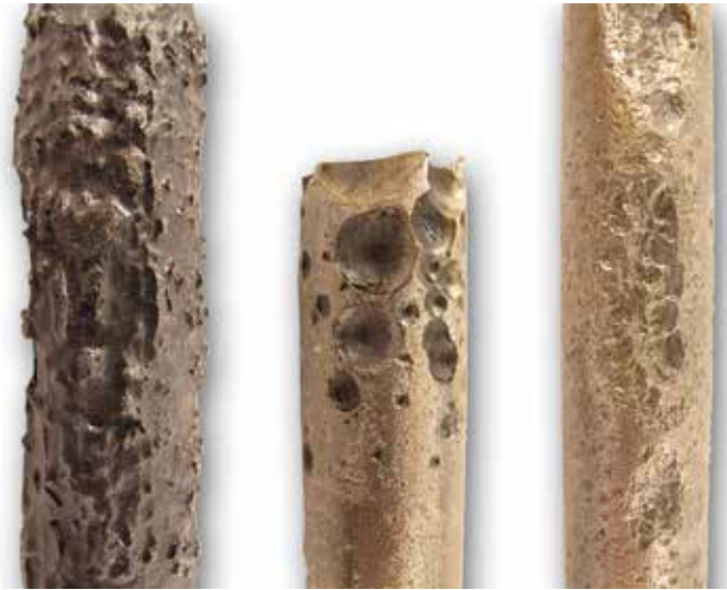
Examples of sucker rods, eaten away by corrosion.
