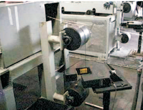
Precise laser monitoring of in-house wire-forming and annealing operations provides the necessary tolerances to wrap directly on the base pipe.
