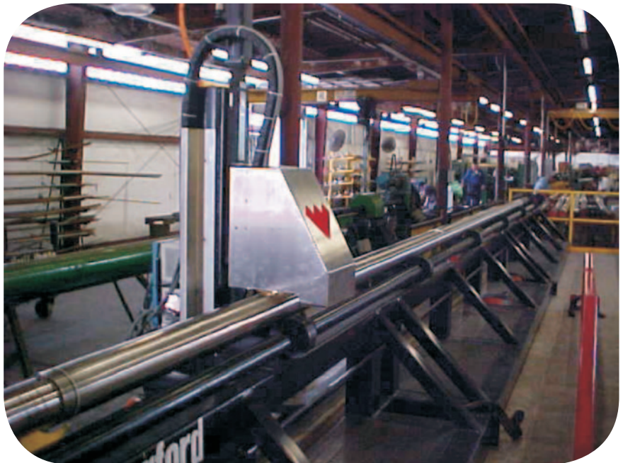
Camera and sensor measure each gap to ensure required tolerance.
