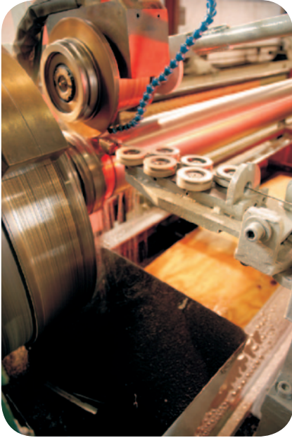
Wire wrap is automatically fed onto base pipe.
