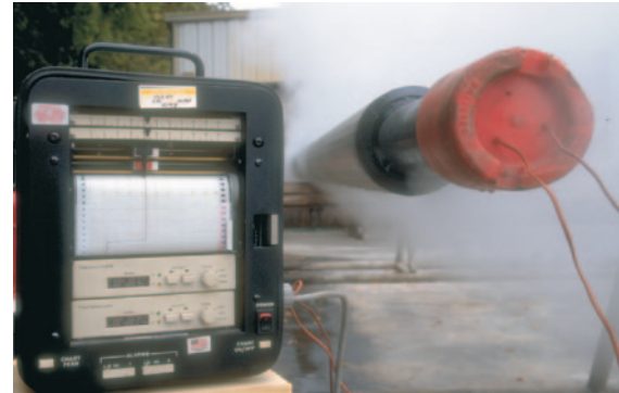
Process controls ensure consistent steam curing.
