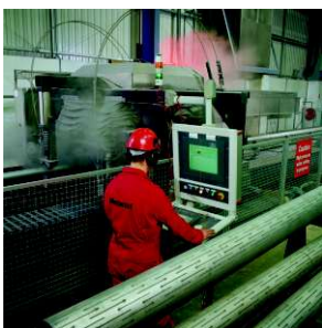
Automated High-Pressure Water Jet Slotting
