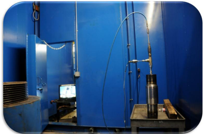
FloReg ICD sample prepared for burst test.
