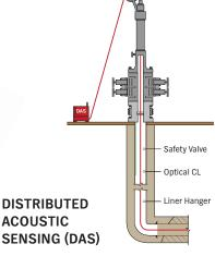
Produce real-time compressional and shear-wave measurements along the optical fiber. Also monitor injections so that treatments reach intended zones. Fiber-optic sensors also process vibrations and translate them into usable datasets.
