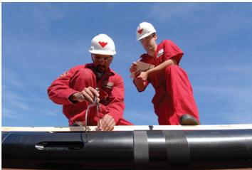
The well screen has been a key component of sand-control completion systems, either as an integral part of the gravel pack or as a stand-alone provider of sand control.
