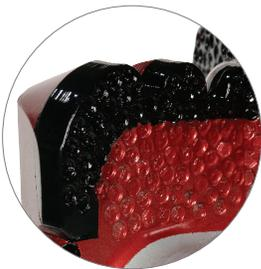
**6-mm round, thermally stable polycrystalline (TSP)** pressed into the aluminum provides a durable cutting structure. Small cutters are easily drilled out and removed from the hole with drilling fluid.
