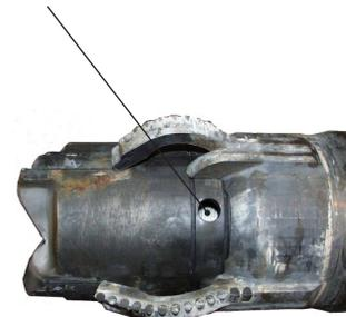
**Displaceable blades** enhance cutting efficiency, rate of penetration, and durability saving time and reducing hole problems.
