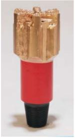
The crushed tungsten carbide used to dress these mills consists of carefully sized, high-grade tungsten carbide particles in a tough matrix. The matrix readily bonds to the mill body and holds the tungsten carbide particles in position as a cutting surface.
