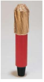
Weatherford *CustumCut* milling- or cutting-grade inserts are available in various configurations and geometries. Our advanced mill engineering and certified welders ensure a consistent and durable cutting structure on every mill and rotary shoe we produce.
