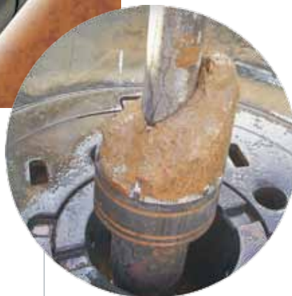
The FJB coming out of the well with solid drilling fluid on top.
