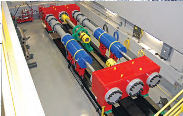
Our 3.1 million-lb test frame is housed in one of the bunkers.
