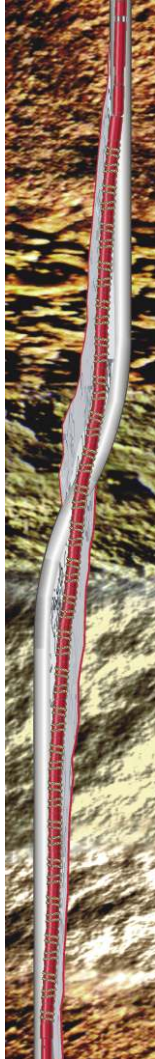
2. Severe dogleg broached
