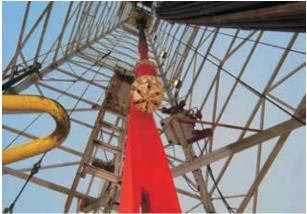
The QuickCut casing exit system is designed for efficiency, which reduces the time and cost needed for sidetracking and for extended-reach, horizontal, and infill drilling. Our QuickCut casing-exit technologies combine a single-trip, full-gauge milling system with a single-angle concave that incorporates multiple anchor options.
