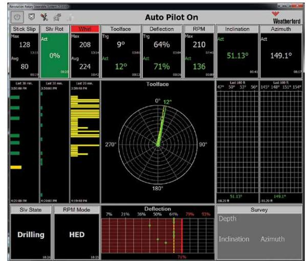
The Revolution RSS rig-floor display shows real-time drilling parameters including whirl, stick slip, and toolface angle. Operator stakeholders can also view real-time data visualizations remotely.
