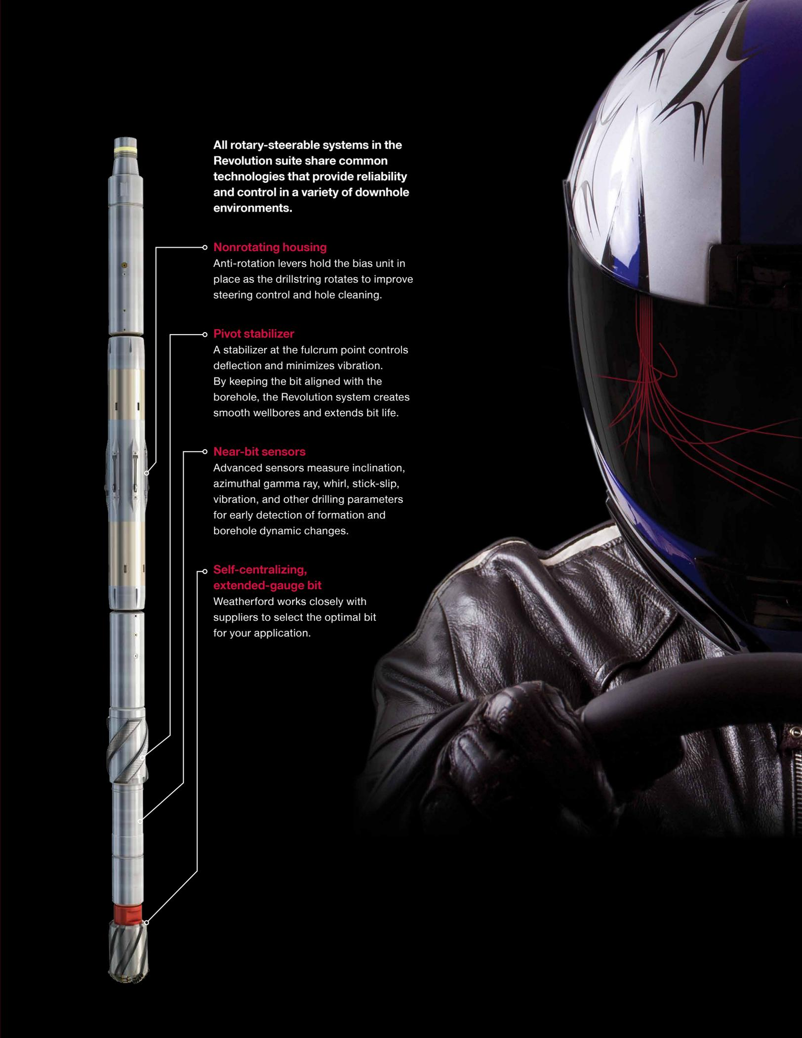
All rotary-steerable systems in the Revolution suite share common technologies that provide reliability and control in a variety of downhole environments.
