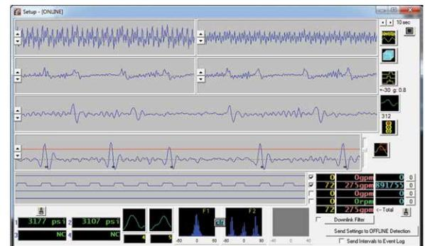
Mud-pulse telemetry is used to transmit operational data between the RSS and the surface. Our proprietary software receives, filters, processes, and decodes the raw pressure pulses into data, which is then displayed in real time.
