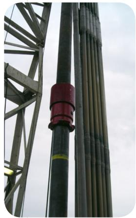
The casing head is integrated into the last joint of casing and runs through the rotary table for maximum installation efficiency.
