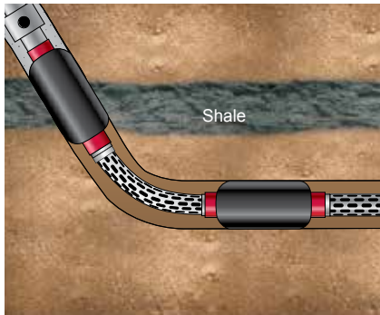
Location: Colombia Solution: BULLDOG ACP annulus casing packers
