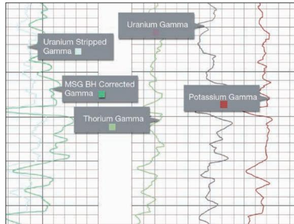
Gamma graph results with Weatherford Compact spectral gamma ray tool
