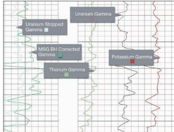
Gamma graph results with Weatherford Compact spectral gamma ray tool
