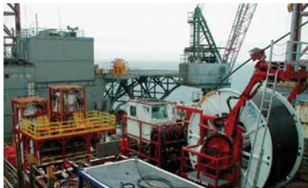
Offshore coiled-tubing equipment meets small footprint requirements.
