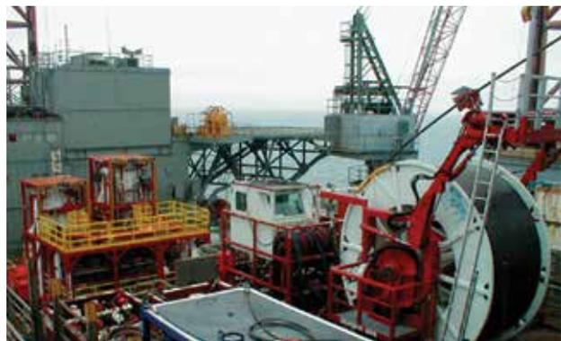
Offshore coiled-tubing equipment meets small footprint requirements.
