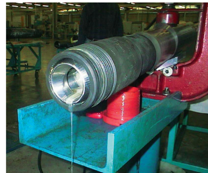
After running a standard valve inside the damaged nipple, Weatherford could not prevent the hydraulic oil from leaking.
