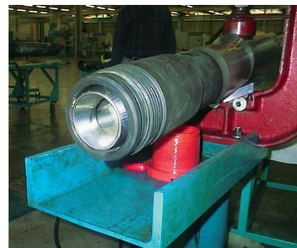
Installation of a Renaissance WDB SSSV solved the problem. Even with such severe sealbore damage, the valve held 6,500 psi (44.8 MPa) in the control-line pressure and 7,000 psi (48.3 MPa) (nitrogen) in the tubing.
